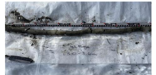
Figure 3. Core recovered from 3.0 to 3.6 meters depth.
